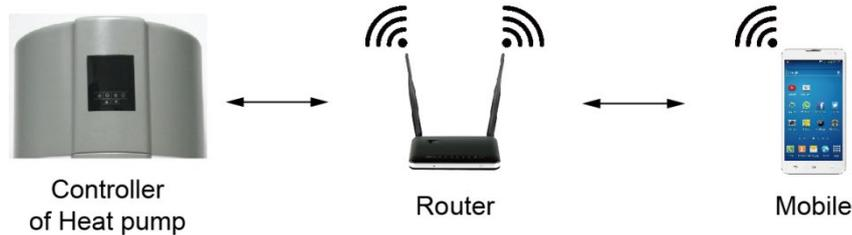
Power on the heat pump unit, and keep pressing the timer button and the increase button at the same time for 5 seconds. The SET
