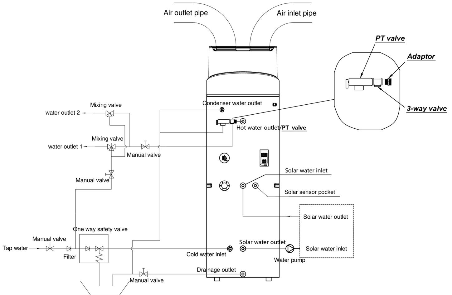
**Note:** Solar heat exchange coil is optional.
