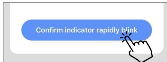
Notes: when the icon of set flashes quickly, it mean the controller is in the Wi-Fi mode. When it flashes slowly, it means the controller is connecting with the App. During the connection, if the icon of set is extinguished, it means the App connection with the unit is finished.
